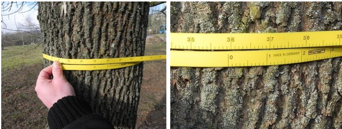
Figure 9. DBH measurement with diameter tape (here 35.9 cm).
