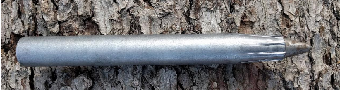
Figure 6. Example of an iron marking pole (25cm) for marking the plot center and corner points.
