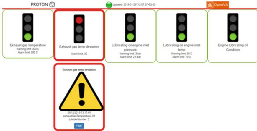
Fig. 13.9 Visual dashboard from a DataBio pilot on fishery. The dashboard shows information and alerts about the status of the fishing vessel's engines
